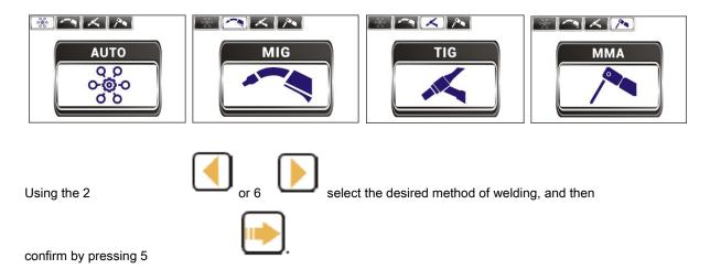
**AUTO mode** - setting synergistic. The user selects the basic welding parameters such as type of material, the plate thickness, the diameter of the welding wire. Other parameters of the device selects automatically uploaded using the base program.
