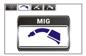
In MIG mode you yourself shall subsequently setting all welding parameters. The system prompts the selection of the optimum welding parameters indicating the adjustment of the plate thickness of the material (see table - set the wire feed speed). This information suggests the user to correct settings made. Depending on the style of welding (forced position, welding current rapidly with a higher intensity of slower or lower current density), the settings may require slight adjustment by the user.
