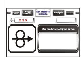
Set the minimum speed of the wire feeder.
