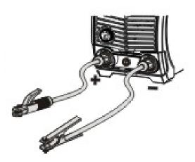
Welding cables and connect the mass to the corresponding output jacks welders, according to the manufacturer's recommended polarity of the electrodes, which intend to weld.
