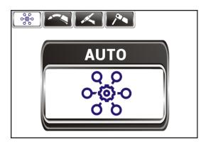
In the AUTO mode, a user makes a selection of only the basic welding parameters such as type of material, the plate thickness, the diameter of the welding wire (available 0.8 mm, 1.0 mm and 1.2 mm). Other parameters of the device selects automatically uploaded using the base program. **AUTO mode only allows continuous welding current**
