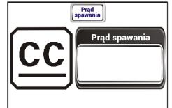
TIG welding is an optional extra. You can only adjust the welding current.
