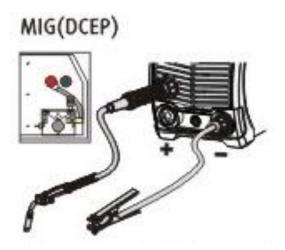
To choose the correct polarity welding as shown above.
