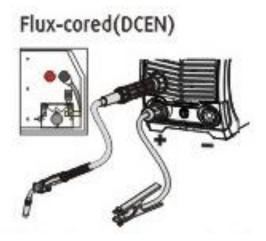
Plug current welders connected to the negative - ( EURO) mass holder connected to the negative +
