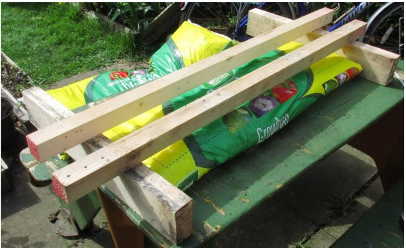
You will need to mitre the ends of the boards to 45° for the boxes. I have set the circular saw up to cut at 45° and I have a length stop in-place so the boards are all the same angle and length when cut, but this can be done manually with some careful measuring and the use of a mitre block and tenon saw (available from DIY outlets). I have chosen 37.5cm or about 15" height for these boxes which works out at 5 boards high.
