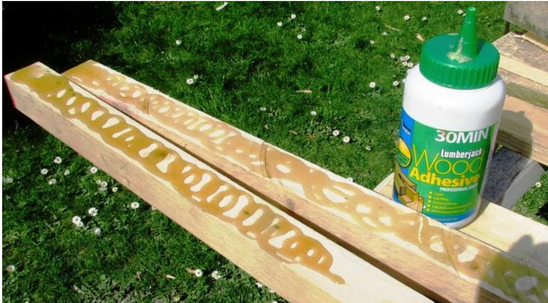
The timbers require only light but firm clamping; too much clamping force can be worse than no clamping at all as it can squeeze the glue out of the joint. After 24 hours the glue will have fully hardened and you may release the clamps, scrape and sand off the excessive dried adhesive, and cut the timbers to length: approx 16" or 40.5cm.
