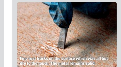
Fine rust tracks on the surface which was all but dry to the touch. The metal remains solid.
