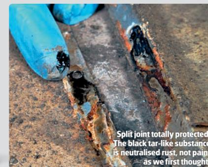
Split joint totally protected. The black tar-like substance is neutralised rust, not paint as we first thought.
