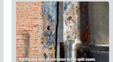
Hardly any hint of corrosion in the split seam.
