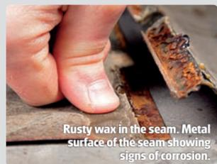
Rusty wax in the seam. Metal surface of the seam showing signs of corrosion.
