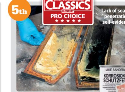
**5th** Lack of seam penetration self-evident.
