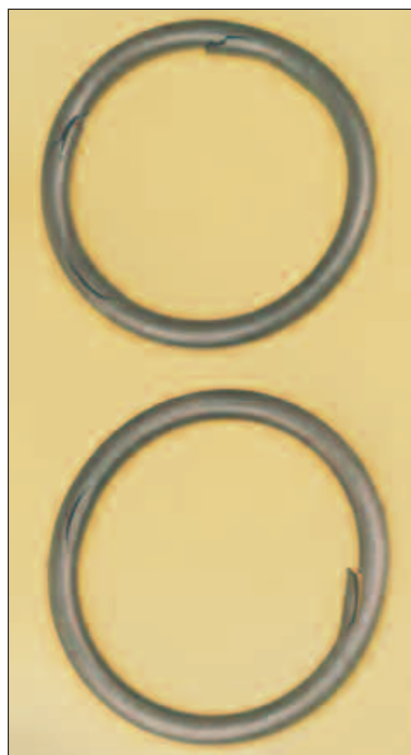
'O' rings after explosive decompression.
