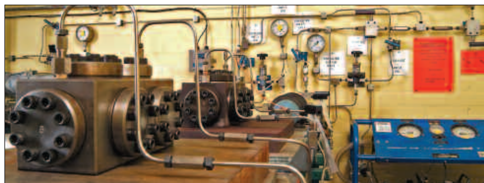
James Walker's eight-flange explosive decompression test rigs.
