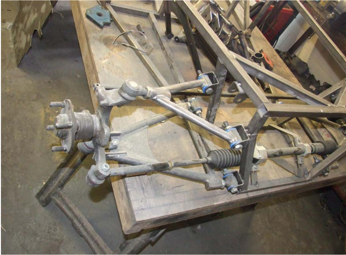
Figure 6 - front suspension geometry
