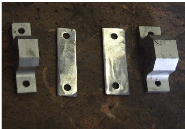
Figure 22: additional 5mm support plates
