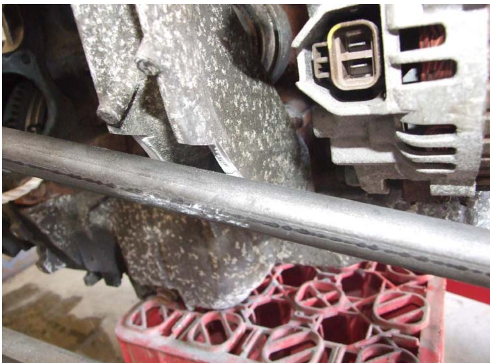
Figure 19: Steering Column Route
