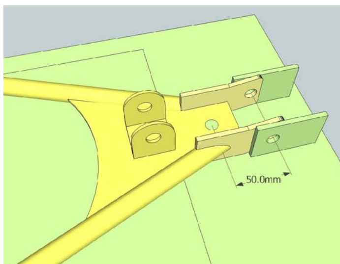
Figure 26: Front lower wishbone ball joint hole spacing
