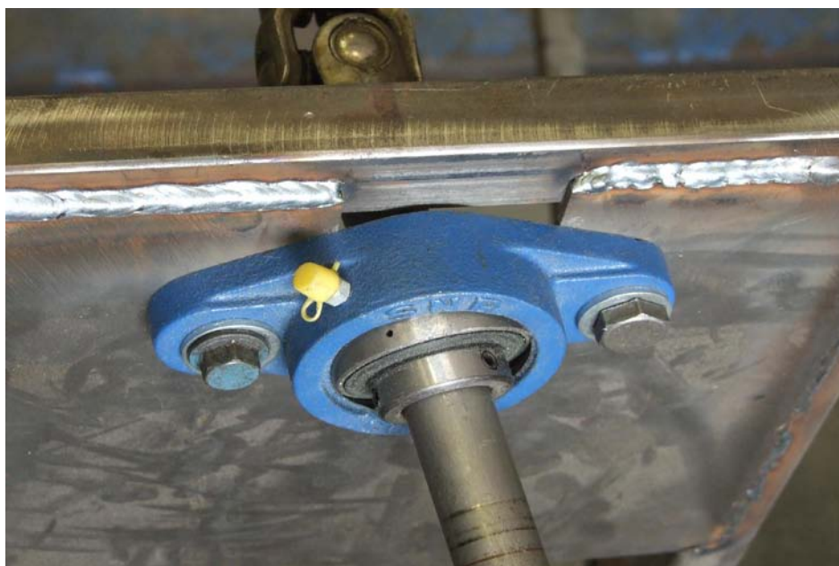
Figure 19: Steering support bearing
