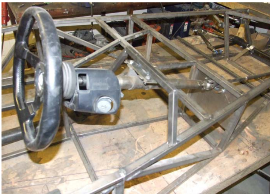
Figure 177: Mx-5 Steering column arrangement
