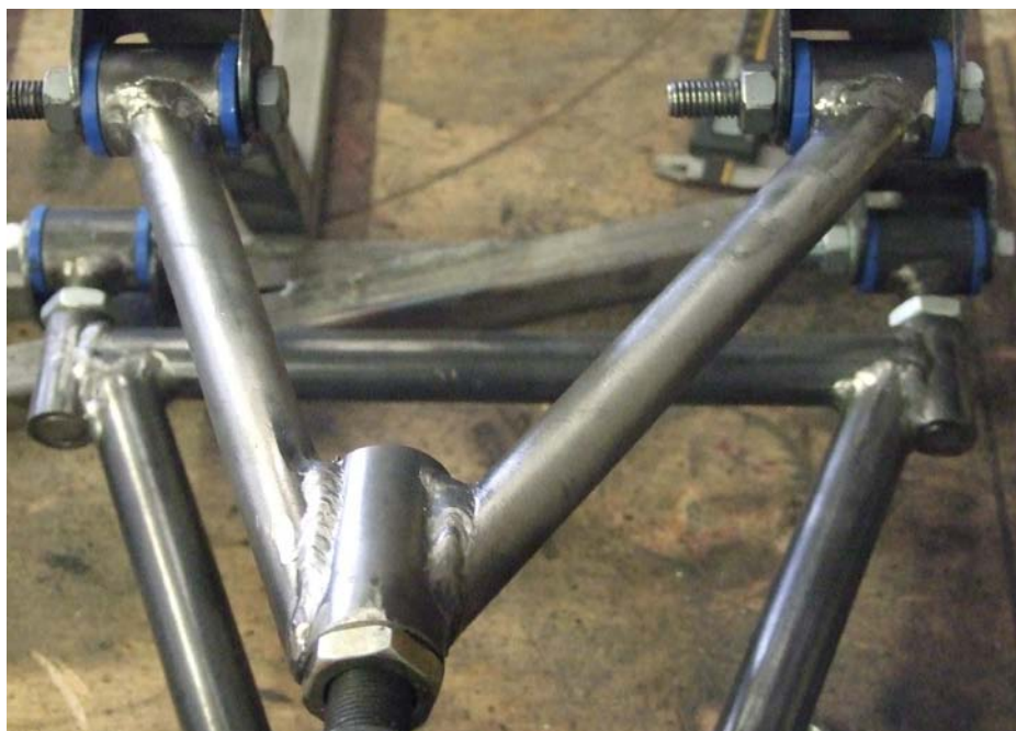
Figure 25: front upper wishbone fitting
