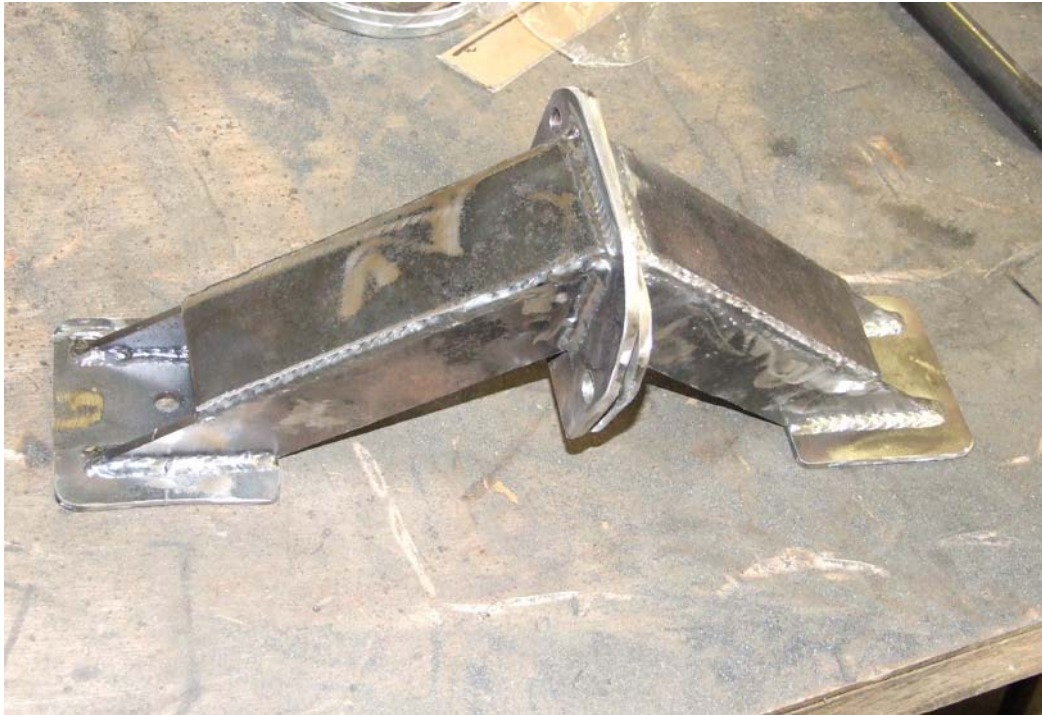
Figure 21: Engine Mounts
