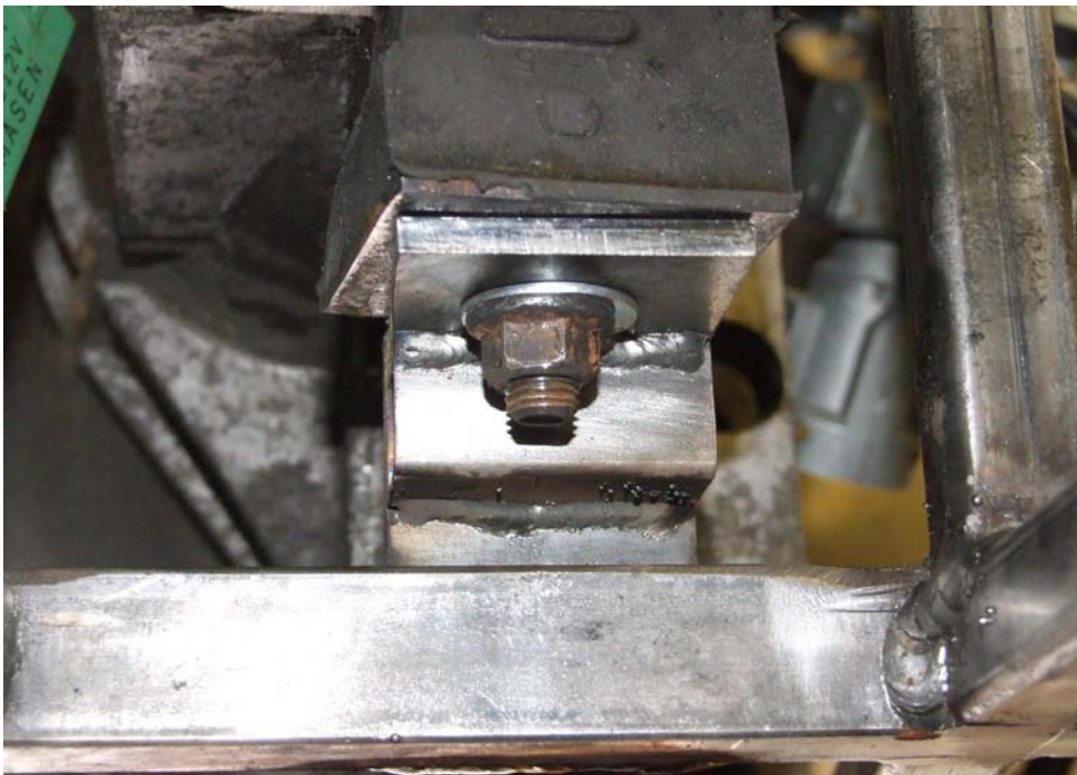
Figure 40: Gearbox Mount
