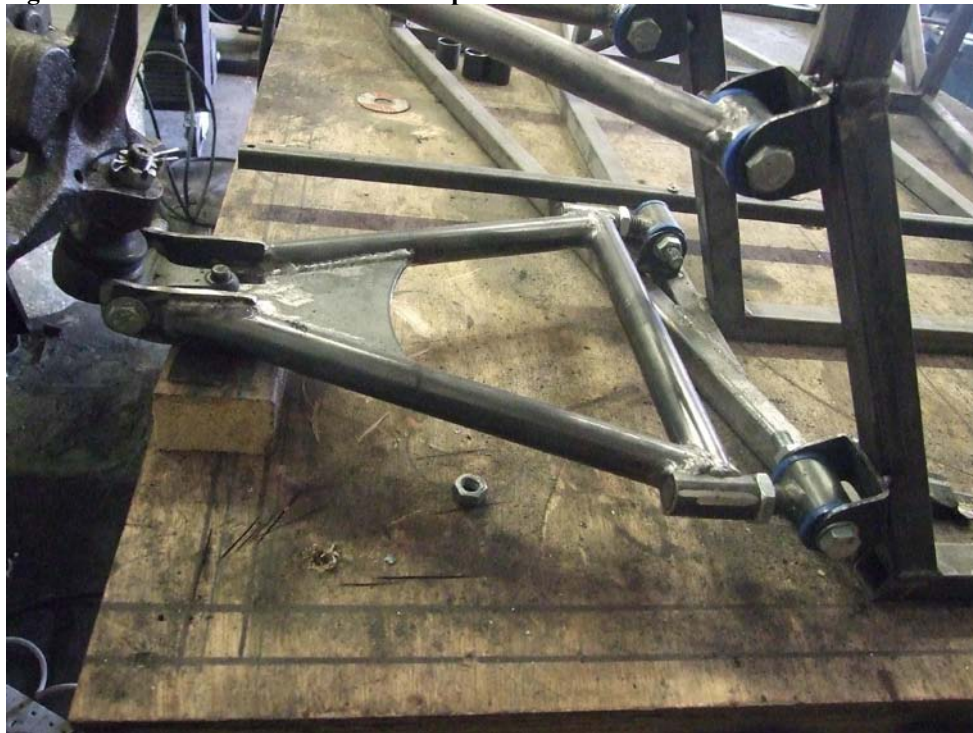
Figure 32: Front lower wishbone fitting
