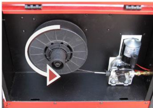
Figure 1. The direction of rotation of the reel of welding wire (illustrative photo)
