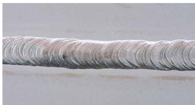
TIG seam, root side, with root protection
