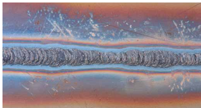
TIG seam, root side, no root protection
