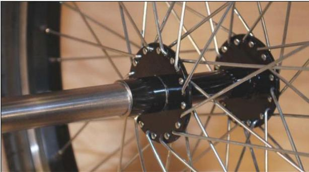
Figure 94 – Outer axle spacer installed
