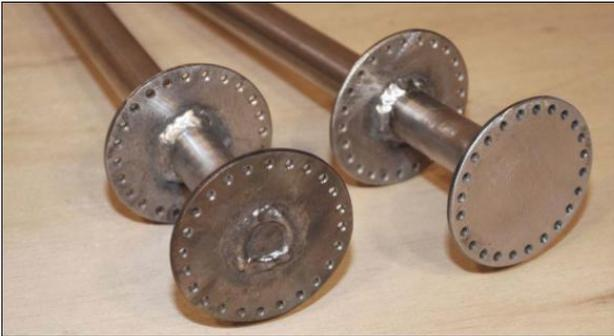
**Figure 89 – Weld both sides and clean up the face**
