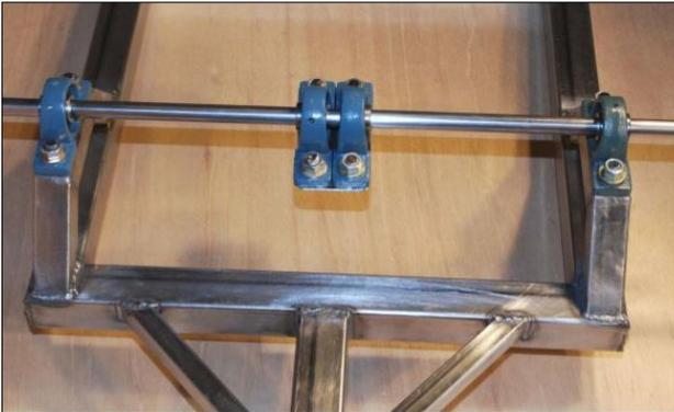
Figure 59 – Install the two center bearings
