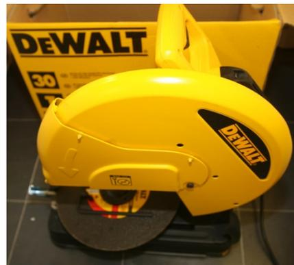
These machines should be set up with adequate space for the length of the material to be cut and with all combustible materials removed from around 1.5 metres to the sides, 3 metres in front and 1.5 metres behind, as shown below.
