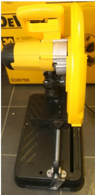
The photograph shows the clamp to secure the material and the guard in its position ready for use. The photograph below shows the side view and the section of the guard which moves as the cut is made.
