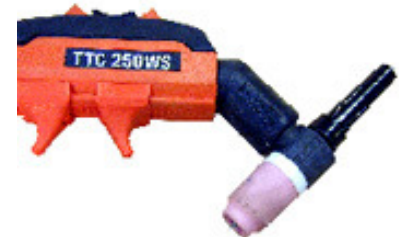
Water cooled model torch TTC 250 WS, with S-neck allow also welding to the negative neck angles ( pipes )
